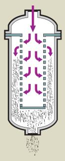
During backwash, triggered by time or pressure differential, a valve switches one station's flow from the inlet header to the drain header and the direction of the flow is reversed in the filter tube, dislodging contaminants from the media surface. The source of the cleaning fluid may be a diversion of process fluids (internal backwashing) or an external source (external backwashing).
