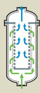
Process liquid flows into the housing inlet at its base and passes across the filter media from the outside inward. Because of this flow path, contaminants collect on the outside of the filter element slowly forming a cake, removing smaller particles.
