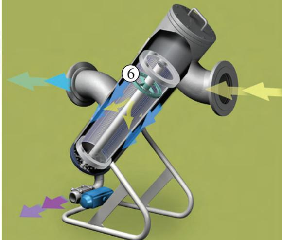
Eaton MCF and MCS operate in much the same manner as DCF units, but add the advantage of a magnetically coupled disc mechanism (6). This unique design eliminates the need for internal seals and reduces maintenance costs.
