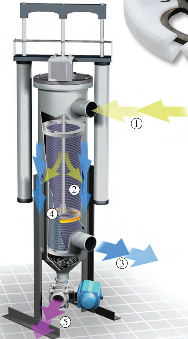
In Eaton's DCF mechanically cleaned filter unit, incoming fluids (1) are channeled from the interior cylinder through a wire screen (2) to the outer cylinder and out the discharge port (3). A cleaning disc (4) travels down and up inside the cylinder to periodically clear the filter screen. Particles are collected at the bottom of the housing where they can be discharged (5).
