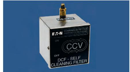
Continuous Cleaning Valve (CCV) is the standard configuration where the cleaning disc continuously cycles, driven by shop airflow. Purge is controlled by a manual valve or push-button.
