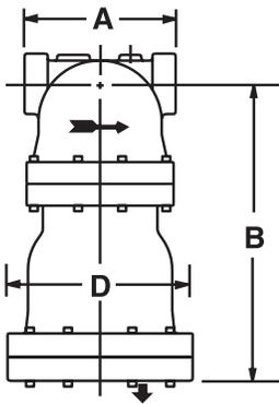
**Dimensions - Type ST & STH - Threaded Inlet & Outlet (in /mm)**
