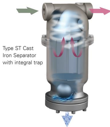
Type ST Cast Iron Separator with integral trap
