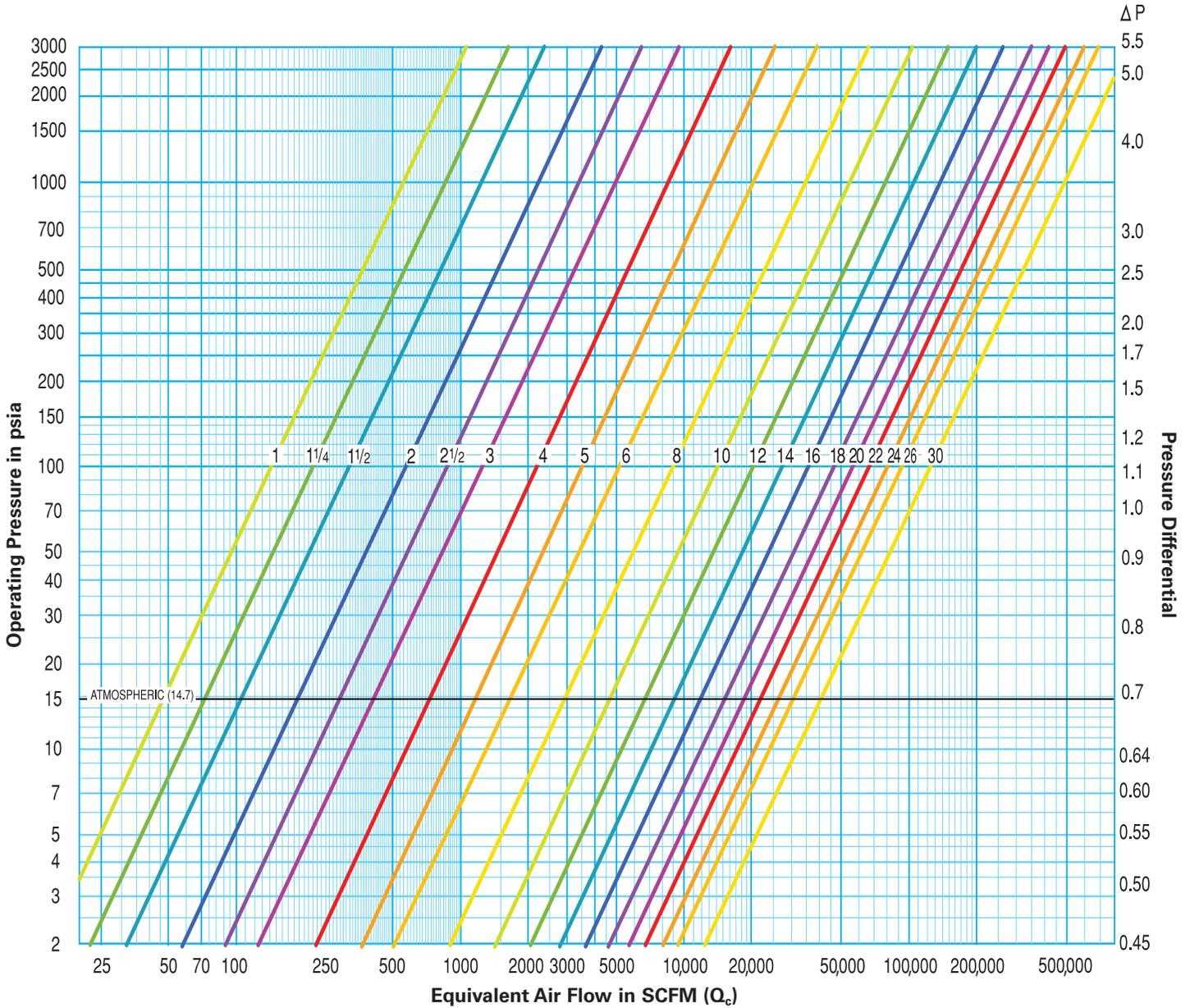
$$\text{Actual Pressure Drop} = \left[ \frac{\text{Application's Equivalent Air Flow SCFM (Q}_c\text{)}}{\text{Separator's Maximum Rated Air Flow SCFM}} \right]^2 \times \text{Rated Pressure Drop (obtain from scale at the right side of this chart)}$$
