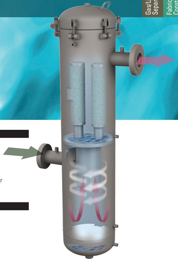
The two-stage Eaton Type TF Separator/Filter removes 99% of all particles larger than 10 microns and is for applications requiring extremely fine entrainment removal.
