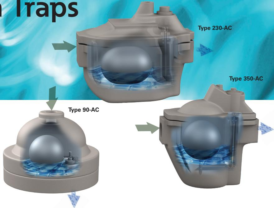
Eaton Float Drain Traps efficiently handle the liquids in the storage tanks and drip points of separators without pressure loss in the line. These traps are capable of removing up to 2800 pounds of condensate per hour and work with pressure differentials from 5 up to 250 psi.
