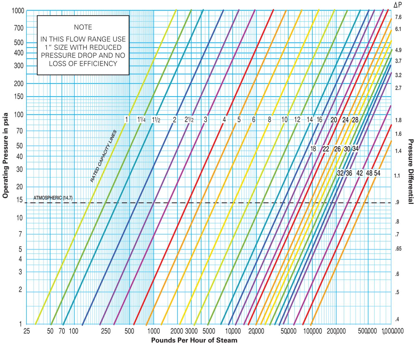
$$\text{Actual Pressure Drop} = \left[ \frac{\text{Actual Steam Flow}}{\text{Rated Steam Flow}} \right]^2 \times \text{Rated Pressure Drop}$$
