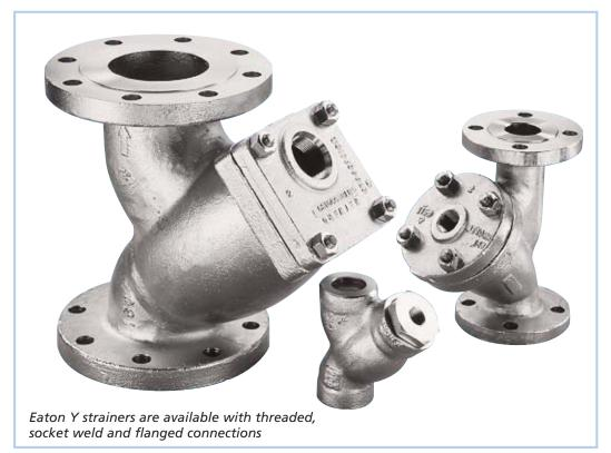
strainers are devices for mechanically removing unwanted solids from liquid, gas or steam lines by means of a perforated or wire mesh straining element. They are used in pipelines to protect pumps, meters, control valves, steam traps, regulators and other process equipment.
